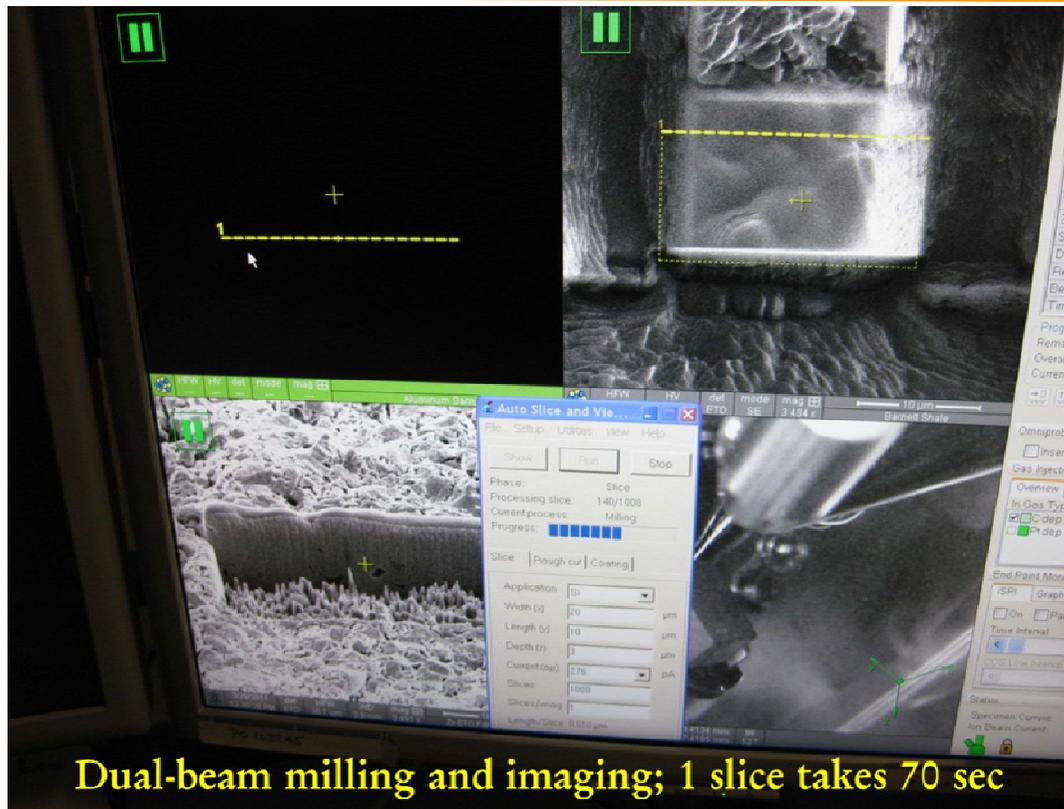
Dual-beam milling and imaging; 1 slice takes 70 sec
