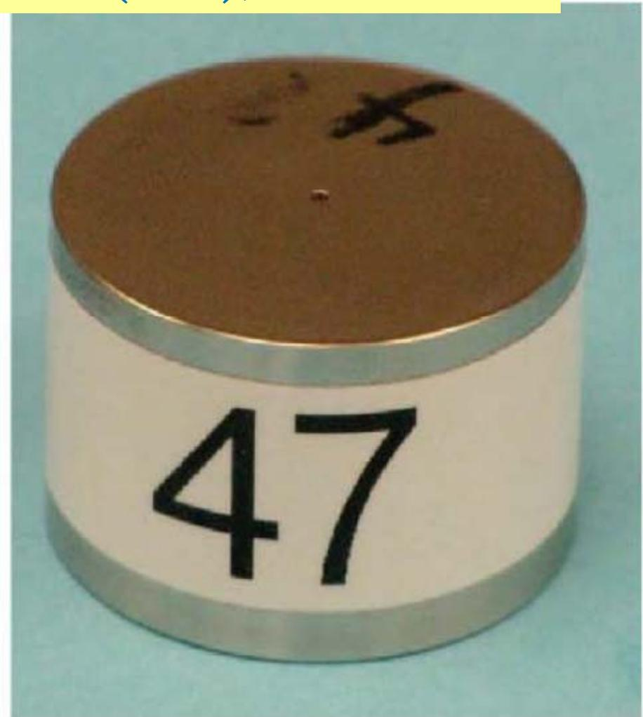
Fig. 3—Capillary-based permeability standard (47- $\mu\text{m}$ -diameter channel).
